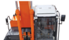
Heat reflective coating on cabin top
