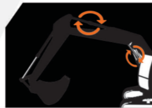
Boom & Arm Regeneration resulting in energy saving
